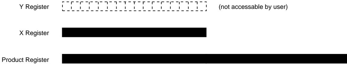
Multiplier operand is fed from X and Y registers (see Architecture). X is visible by instruction, Y is supplied from various source (such as constant, memory, accx).
