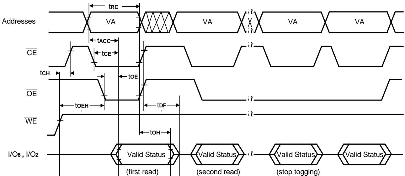
Note: VA = Valid Address; not required for I/O6. Illustration shows first two status cycle after command sequence, last status read cycle, and array data read cycle.
