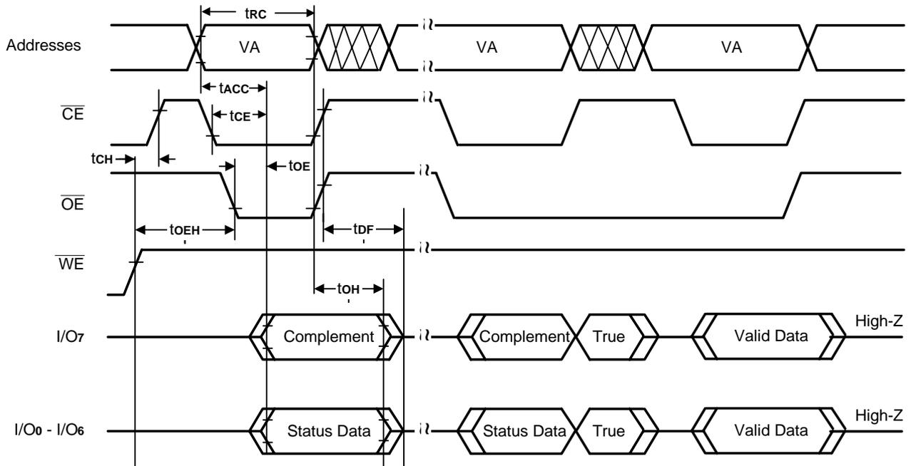
Note : VA = Valid Address. Illustration shows first status cycle after command sequence, last status read cycle, and array data read cycle.
