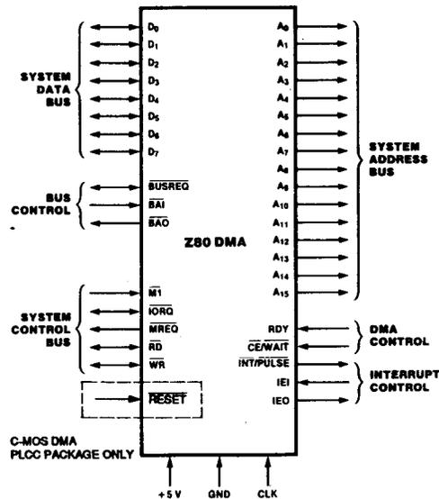
Figure 1. Pin Functions
