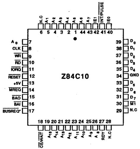
Figure 2c. Z84C10 CMOS Z80 DMA PLCC Pinout
