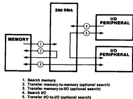
Figure 4. Basic Functions of the Z80 DMA
